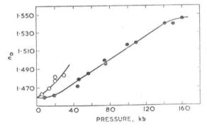
Fig. 1. Refractive index of silica glass measured at atmospheric pressure and room temperature as function of the pressure of the run
